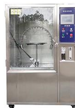
IPX12 IPX34 Water Proof Test Chamber
