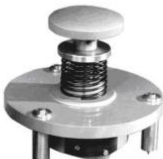
SAMPLER DEVICE OF Flat Crush Test (FCT)
